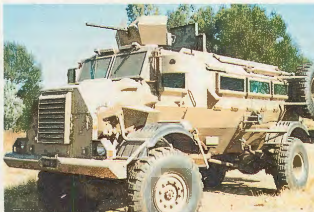
GA1 20x82mm automatic cannon in an internal hand-control mount on the highly regarded South African Casspir Mine-Protected Vehicle.
